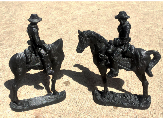
The 2 printed halves were Fused together using SureHold Cyanopoxy Adhesives
