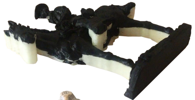
Model Printed with a CubePro Duo in 2 Parts using PLA and Infinity™ Rinse-Away support material
